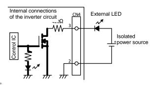
In this case the maximum current flowing through the CN4-3 pin will be 9mA. Maximum voltage that can be applied to the CN4-3 pin is 50V. When using external LED, make sure that these maximum allowable voltage and current are not exceeded.
