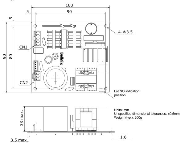
7-1-2. Pin assignment of the PFC circuit board
